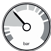
Fig.50 Boiler pressure gauge
